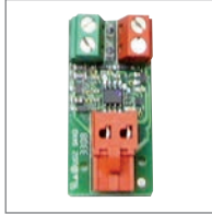
BUS INTERFACE BOARD For traditional photozell connection.
